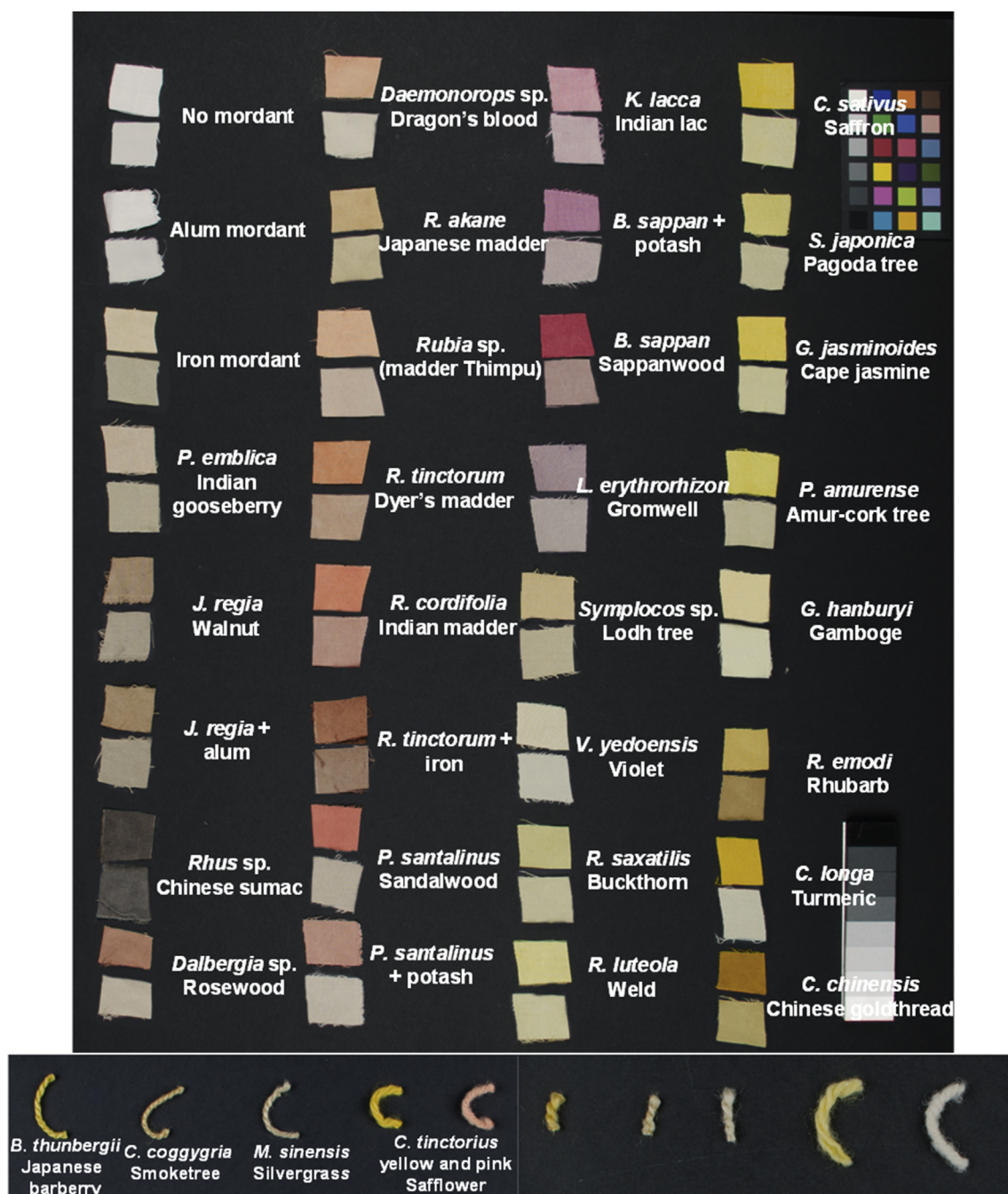
Fig. 1. Image of the set of reference samples under investigation. The samples are shown as pairs: for each pair the upper samples are non-aged and the lower samples are aged. In the low part of the image, the samples on the left are non-aged and the samples on the right, representing a sub-sample of the samples from the left, are aged.
