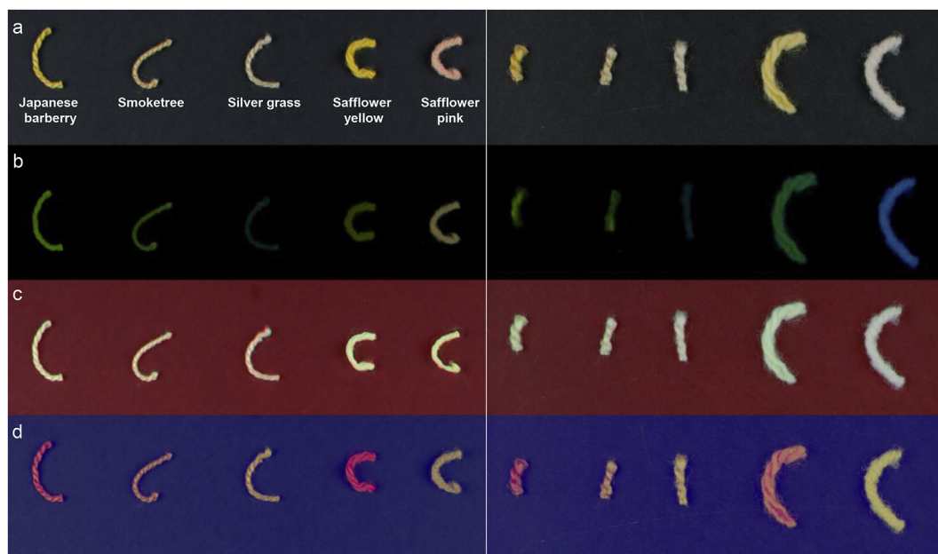
Fig. 5. a) Visible-reflected (VIS), b) ultraviolet-luminescence (UVL), c) infrared-reflected false colour (IRRFC) and d) ultraviolet-reflected false colour (UVRFC) images obtained for the reference samples. The samples on the left are non-aged and the samples on the right are aged. (For interpretation of the references to colour in this figure legend, the reader is referred to the Web version of this article.)
