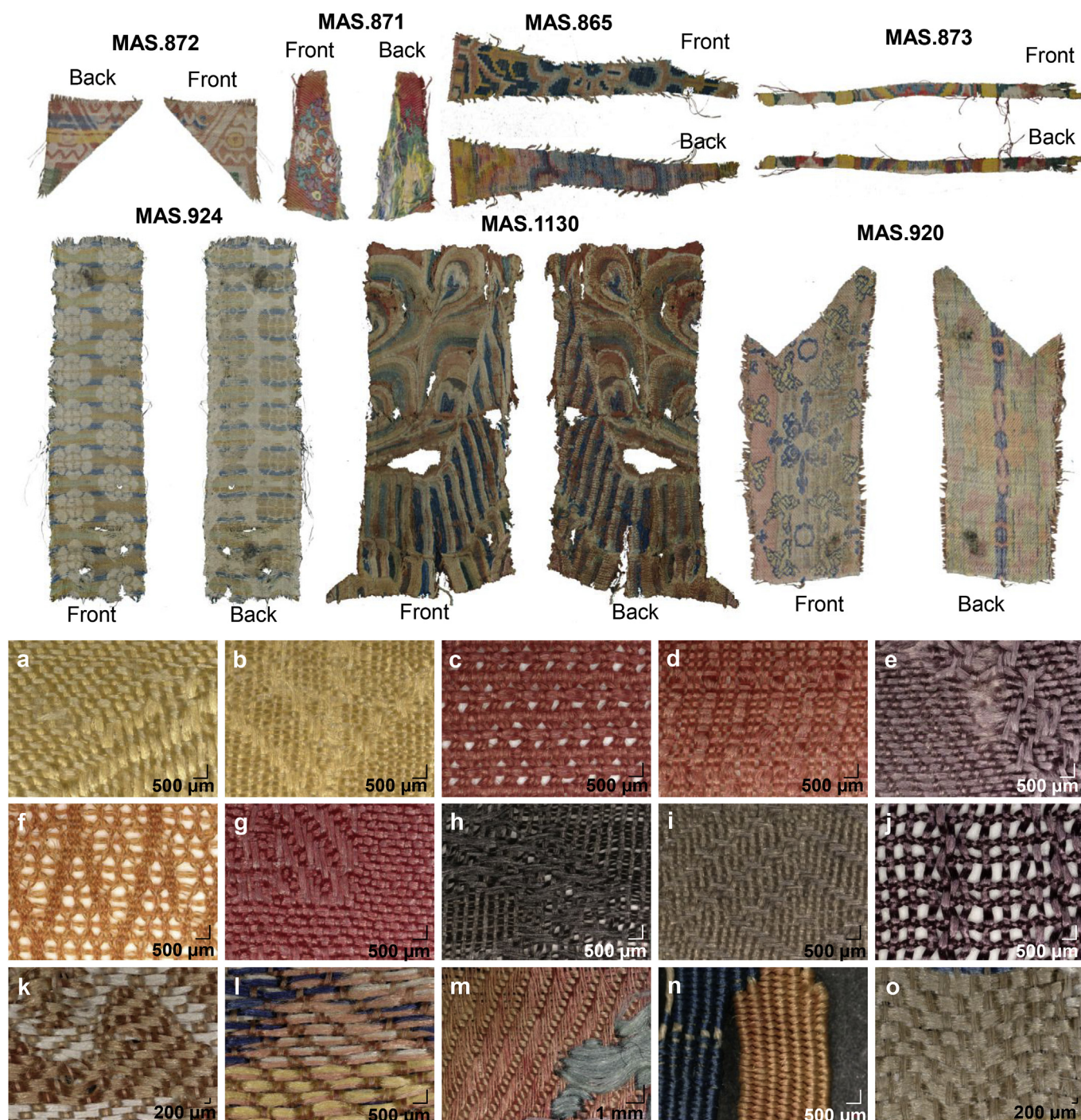
Fig. 1. Top: images of some of the textiles under investigation Bottom: images obtained by digital microscopy showing the variety of weaving techniques: a) MAS.935 twill damask, b) MAS.942 damask on plain weave, c) MAS.954 patterned complex gauze, d) MAS.951 ribbed weave, e) MAS.891 twill damask, f) MAS. 904 patterned complex gauze, g) MAS.934 twill damask, h) MAS.896 damask on plain weave, i) MAS.949 damask on plain weave, j) MAS.900 simple gauze, k) MAS.872 sogdian samite, l) MAS.920 liao samite, m) MAS.871 brocade on twill, n) MAS.906 kesi, o) MAS. 924 double weave.
