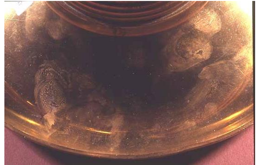
A metal object that has been handled without gloves. Even touching it once is enough to leave a greasy residue!
