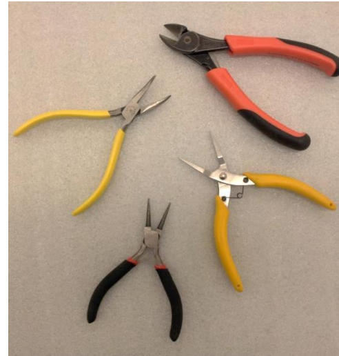
Clockwise from top: side cutters, flat pliers, round nose pliers, pinning pliers
